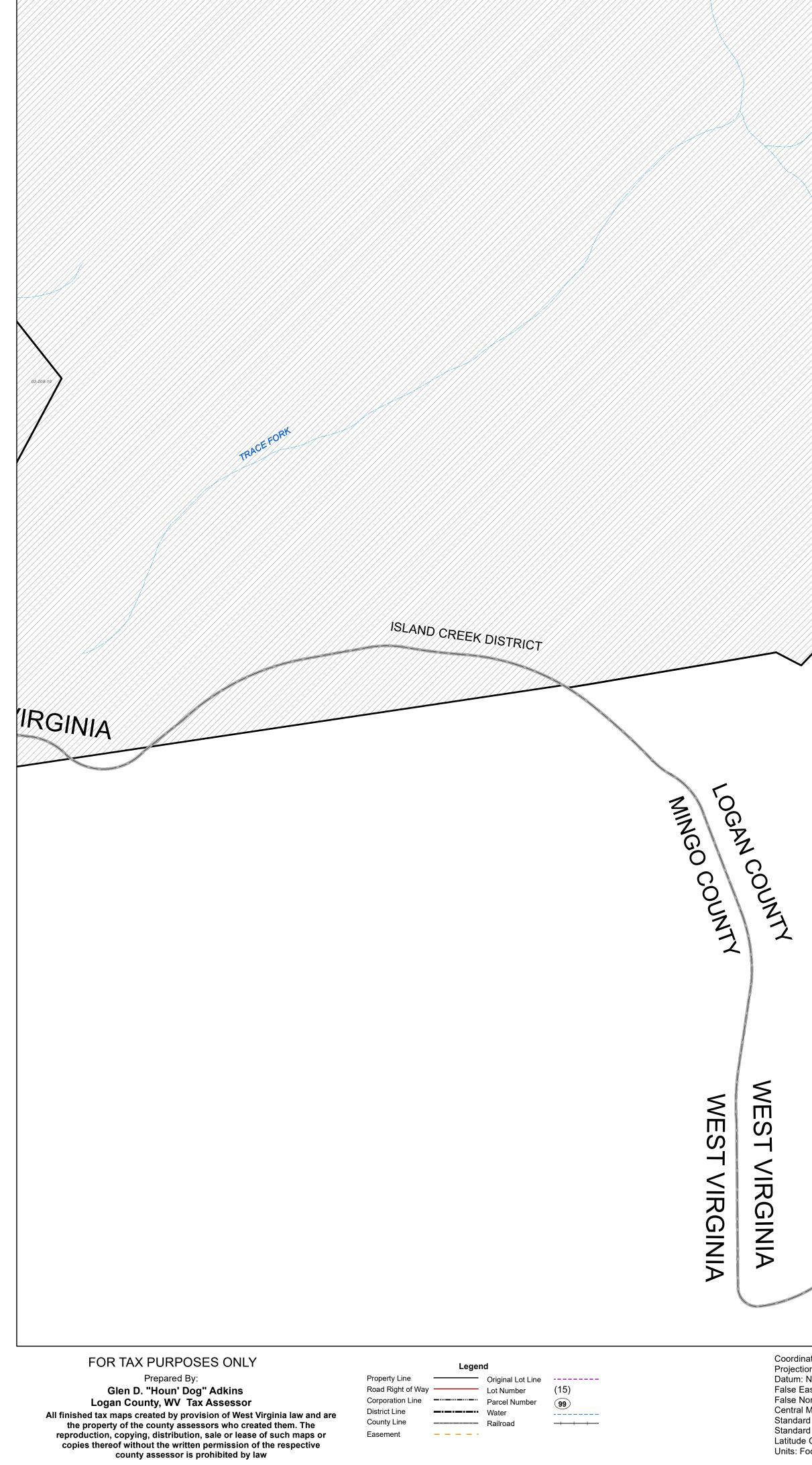
Coordinate System: NAD 1983 StatePlane West Virginia South FIPS 4702 Feet Projection: Lambert Conformal Conic Datum: North American 1983 False Easting: 1,968,500.0000 False Northing: 0.0000 Central Meridian: -81.0000 Standard Parallel 1: 37.4833 Standard Parallel 2: 38.8833 Latitude Of Origin: 37.0000 Units: Foot US
