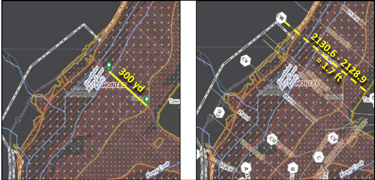
Figure 5. Example of floodway expansion and base flood depth increase in Marlinton viewable on the Risk MAP View of WV Flood Tool
