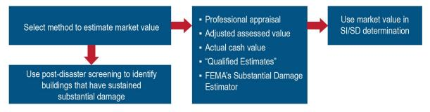
Figure 3. Determining the market value (from FEMA P-758, Figure 4-3)
