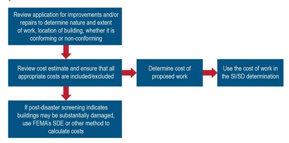
Figure 2. Determining the cost of the work (from FEMA P-758, Figure 4-2)
