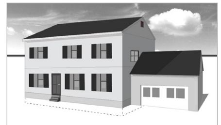
Subgrade crawlspace with attached garage
