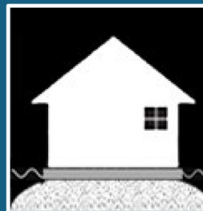
Raised Foundation on Slab or Fill
