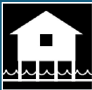
Open Foundation (Columns, Posts, Piers, Piles)
