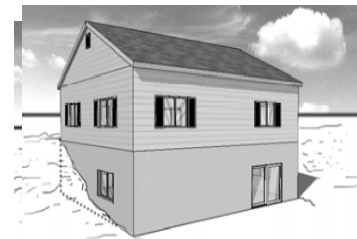
Elevated with Enclosure Not on Post, Pile, or Pier (Solid Foundation Walls)
