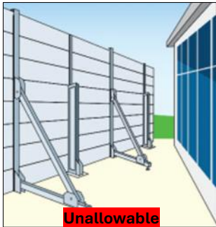
Example of unallowable shield configurations (non-opening barrier due to nonlinearity) protecting an unallowable non-flood opening (permeable curtain wall) for new construction and substantial improvements.
