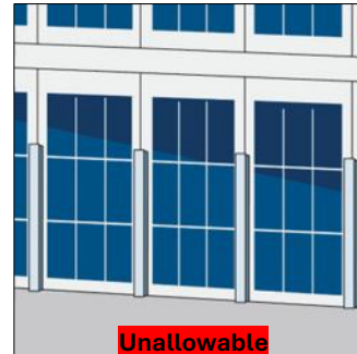
Example of a shield configuration protecting an unallowable non-flood opening (permeable curtain wall) for new construction and substantial improvements.
