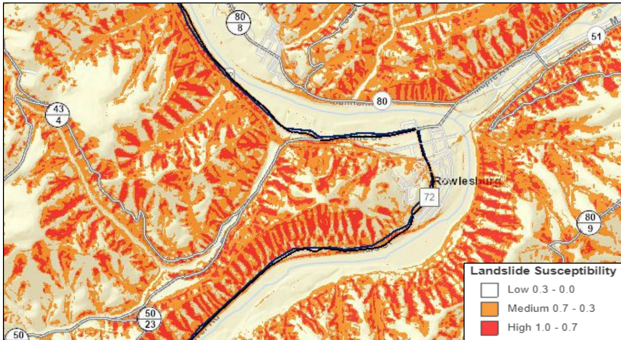
Figure 9. Landslide Susceptibility near Rowlesburg, WV in Preston County. Notice high and medium landslide susceptibility areas along WV-72. Data can be accessed on WV Flood Tool
