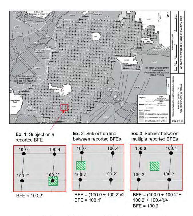
Figure 11: Example of FIS Grid Insert and Calculations to Determine a BFE
