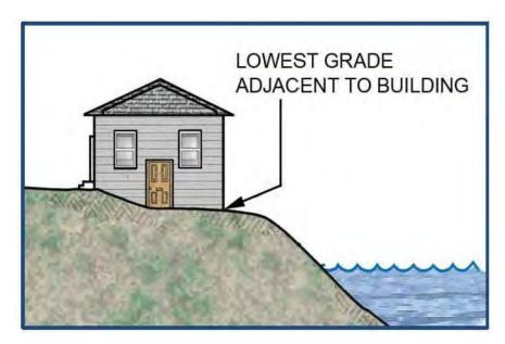
Figure 1: LAG - Lowest Ground Touching a Structure
