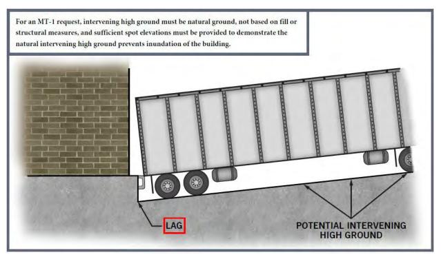
Figure 23: Use of Intervening High Ground – Loading Dock
