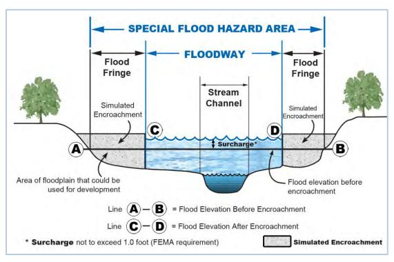
Figure 14: Regulatory Floodway Schematic
