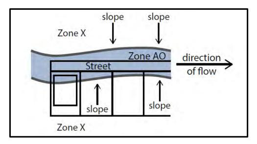
Figure 15: Zone AO SFHA Contained Primarily in Street
