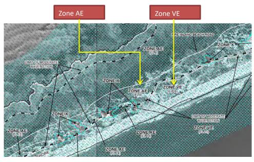
Figure 13: Snapshot of FIRM with Coastal Zones Identified
