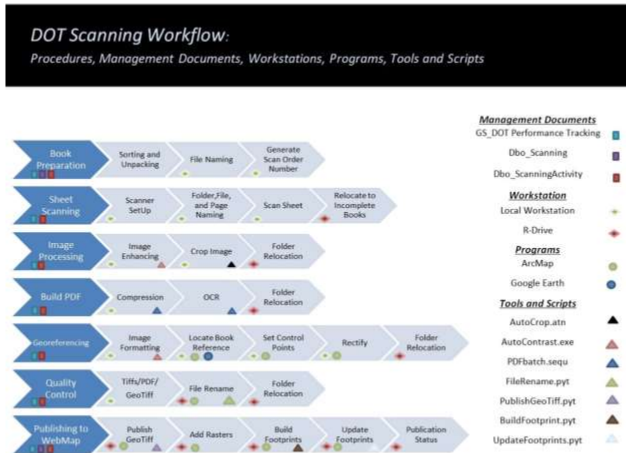
Figure 1: DOT Scanning Workflow
